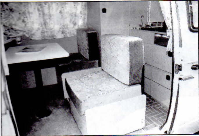
Entrance from side door, with rear seats pulled apart to provide two singles (seat box nearest camera is mounted on runners for easy sideways movement, locked by a bolt).
