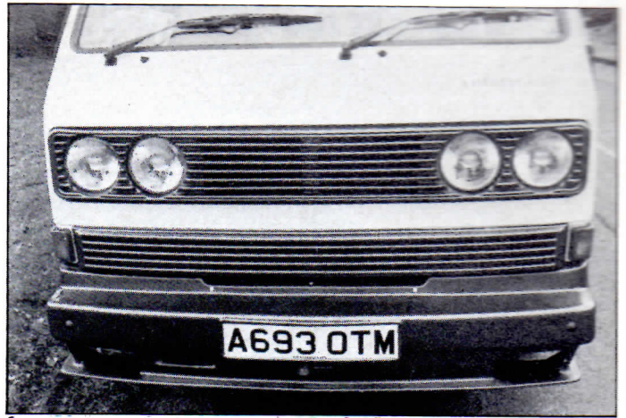
Elite pack consists of ivory wheel discs, wide front grilles with four headlamps and matching bumpers with front spoiler.
