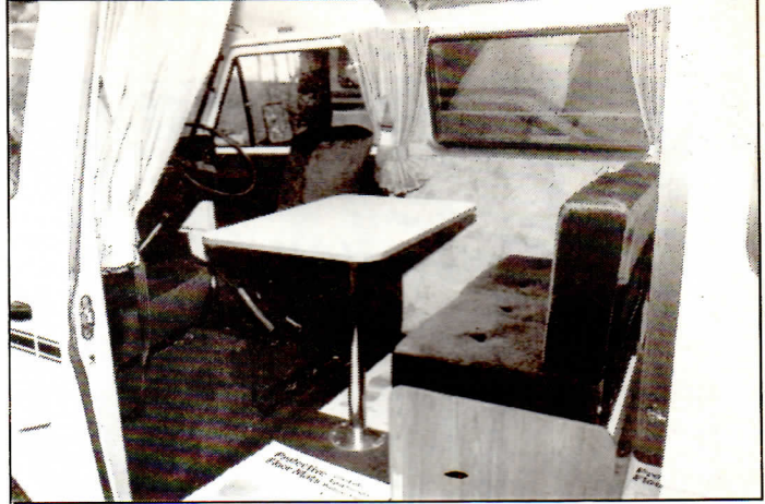
Dining room at front end. Reversible cab seats allow four to sit at table. Front and rear seats recline fully to make twin single beds extending into the cab — left hand passenger seat slides across to nearside.
