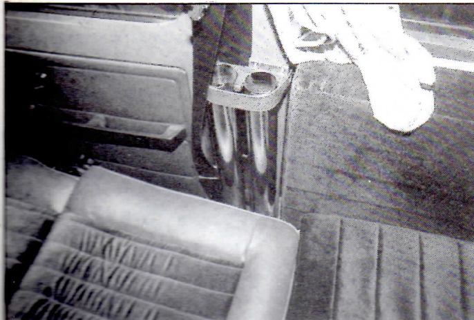
TT number 14: twin table legs are stored in rattleproof housings by side of driver's seat (here reclined to make single bed). Back-rest of this seat is firmly supported when lowered and may therefore be used to provide extra sitting accommodation on site.
